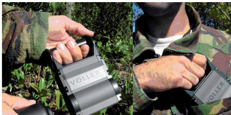
A prototype V100 fuel cell for use in military applications (Courtesy of Voller)
