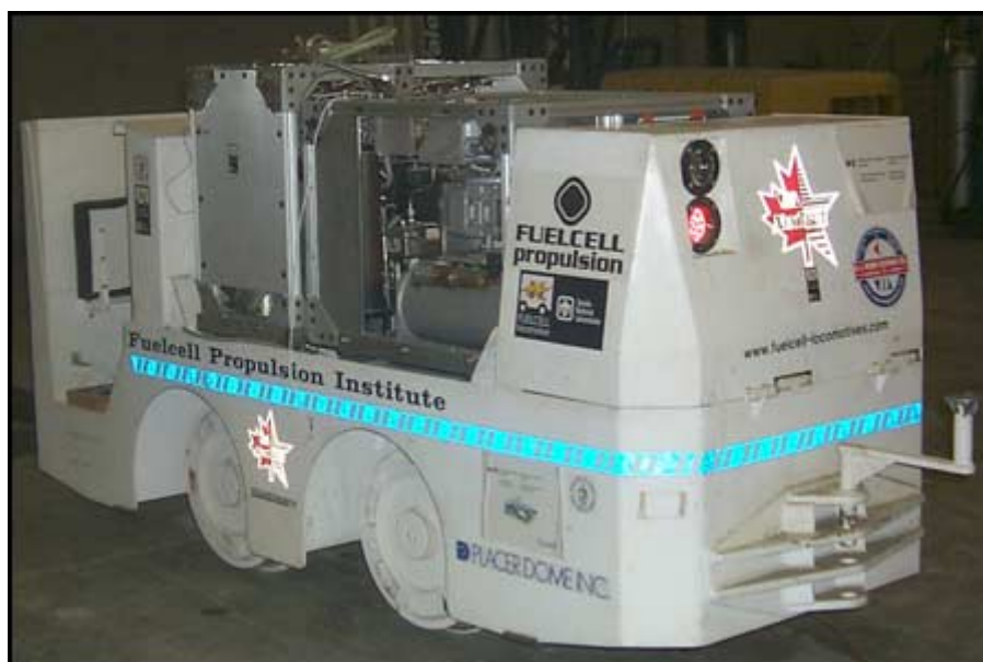
Fig1, Fuel Cell Locomotive under ground. Source: Fuelcell Propulsion Institute
