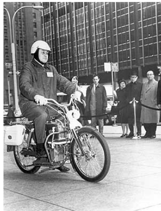
Dr Karl Kordesch of Union Carbide driving his AFC powered motorbike (Courtesy of Smithsonian Institute)
