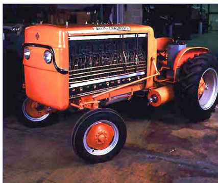
The world's first fuel cell powered vehicle. Allis-Chalmers developed the AFC tractor in 1959.
