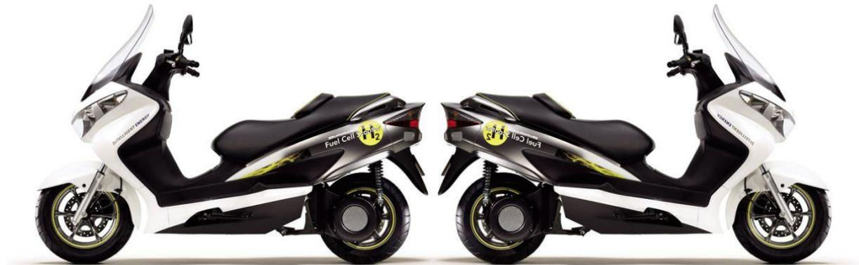
*Suzuki's Intelligent Energy fuel cell powered Burgman scooter (Source: Suzuki)*
